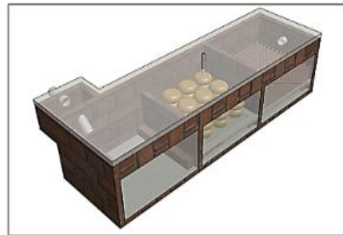
Figure 11. Gravel (3-6mm in diameter) filter materials in the Filter unit
