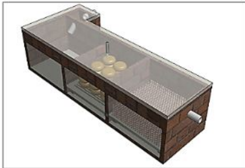
Figure 10. Gravel (3-6mm in diameter) filter materials in the Filter unit
