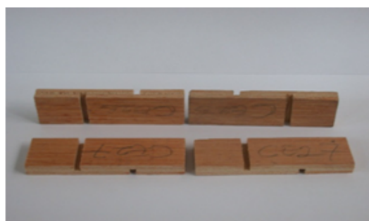
Figure 2. Plywood test pieces for bond evaluation
